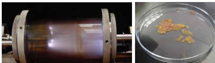
Figure 5. Images of the synthesis of polypyrrole by plasma. Left: the reactor where the synthesis took place; right: thin films obtained at the end of the reaction.
